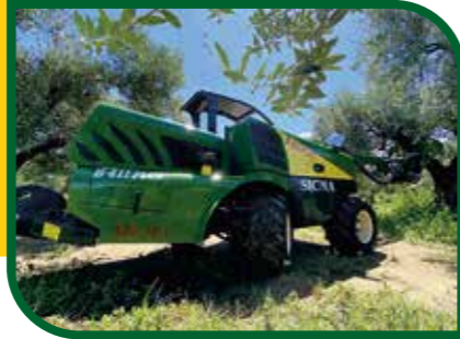
Ponte posteriore sterzante e oscillante Steering and oscillating rear axle
