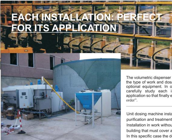
The volumetric dispenser CT-16/360 adapts to the type of work and dosage required with its optional equipment. In order to do this, we carefully study each installation and its application so that finally everything is done "to
