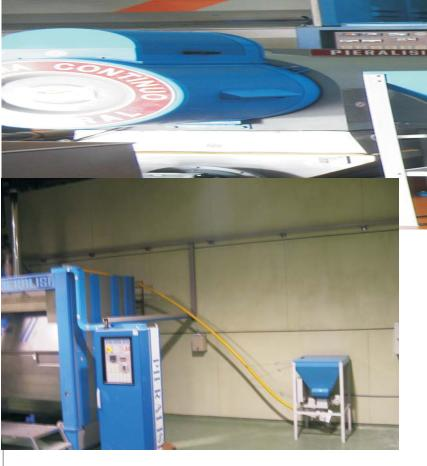
The CT-16/360 volumetric dispenser is a machine capable of carrying out 2 jobs: The dosage of any powder product and the its transport to the receiving machine.
