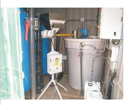
The small size of this DP dispenser means that there is no problem with its set up in very small production plants, even in sheds with very little space. However, the work that it does is industrial and accurate.
